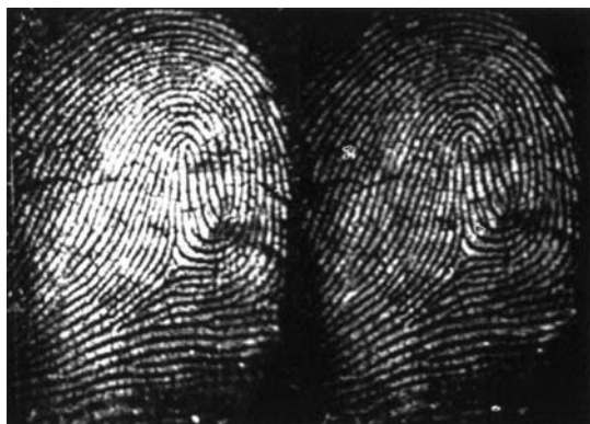
FIG. 11—Two-year-old fingerprint on a white plastic garbage bag after treatment with cyanoacrylate and Basic Red/Basic Yellow stain (observation in the luminescence mode): CONDOR™ (left), Poliview (right).
