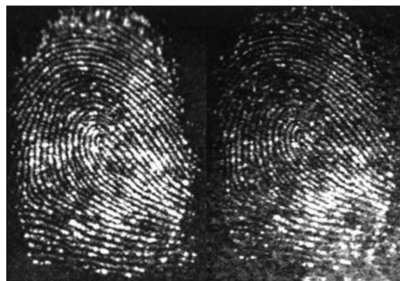
FIG. 9—Fingerprints on paper aged for 19 years and developed with DFO, with observation in the luminescence mode: CONDOR™ (left), Poliview (right).
