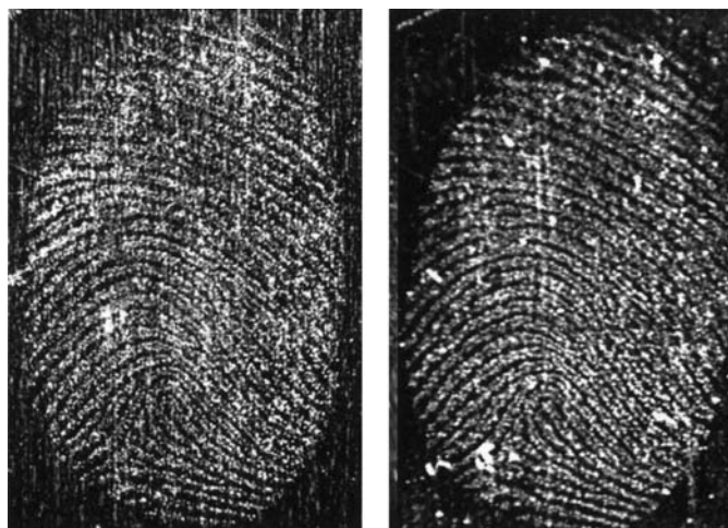
FIG. 2—One-week-old latent fingerprints on a clear plastic sheet: CONDOR™ (left), Poliview (right).
