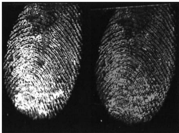
FIG. 12—One-week-old fingerprint on a clear glass slide after treatment with cyanoacrylate and rhodamine 6G (observation in the luminescence mode): CONDOR™ (left), Poliview (right).
